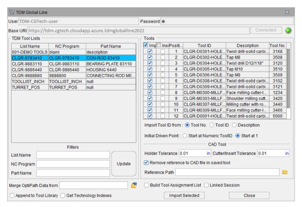
Subsequent activation of the TDM Global Line Interface icon will automatically recall the encrypted User, Password, and Base URI information and populate the appropriate fields. The user only needs to click Connect to use the TDM Global Line Interface.
